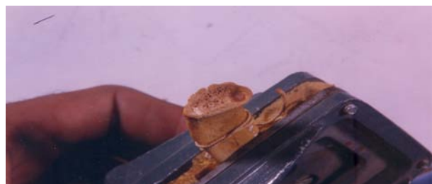
Photograph 2 Showing Increasing Pit Depth with Wide 'U' Shaped Pit Having Brittle and Porous Texture
