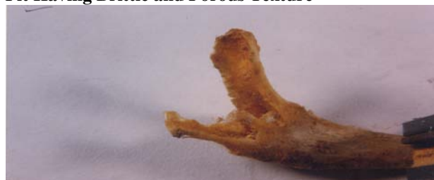
Photograph 3 Showing Still Increasing Pit Depth with Irregular Sharp Rib Having Bony Projections With Incomplete Walls
